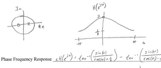
Type of Filtering Operation Lawress Filter
