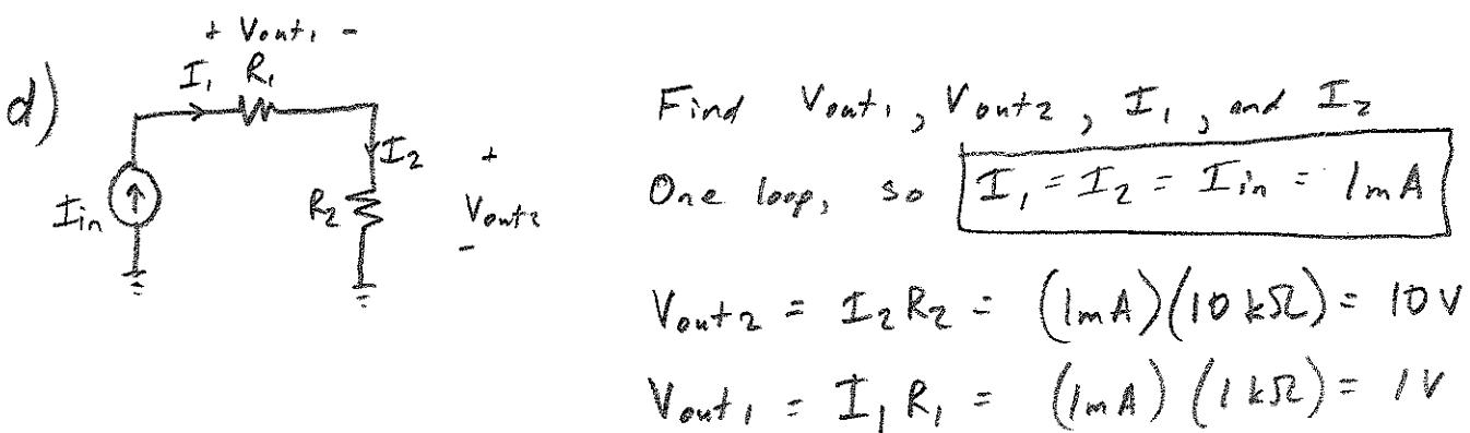
Find  $V_{out1}$ ,  $V_{out2}$ ,  $I_1$ , and  $I_2$
