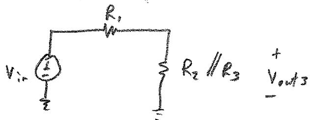
$$I_1 = \frac{V_{out1}}{R_1} = \frac{V_{in}}{R_1 + R_2 // R_3}$$
