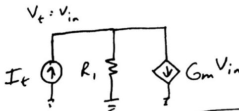
$$\underline{\text{KCL}} \quad I_t = \frac{V_t}{R_1} + G_m V_t$$
