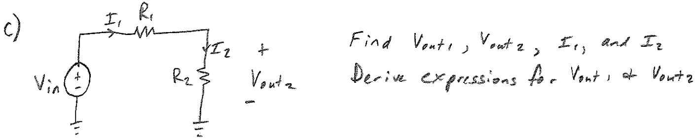
Find  $V_{out1}$ ,  $V_{out2}$ ,  $I_1$ , and  $I_2$
