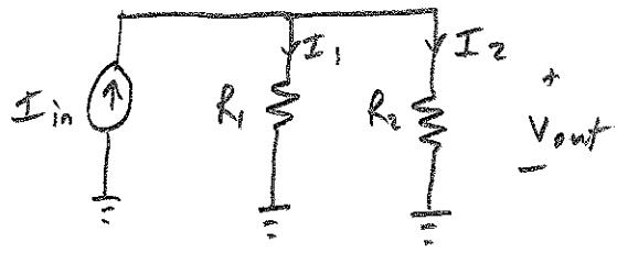
Find  $V_{out}$ ,  $I_1$ ,  $I_2$ Derive the expression for  $I_1 + I_2$
