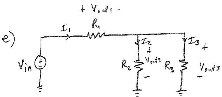
Find the Voltage across each resistor, and also find the current through each resistor
