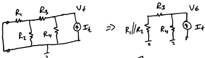
$$V_t = (I_t) [R_4//(R_3 + R_1//R_2)]$$
