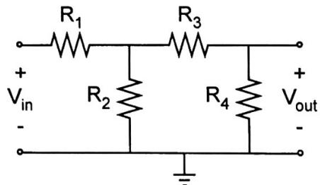
Input Impedance  $\rightarrow$  Apply a test current source at the input while the output floats. Measure the change in the input voltage
