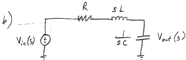
$$V_{out}(s) = V_{in}(s) \frac{\frac{1}{sC}}{R + sL + \frac{1}{sC}} = V_{in}(s) \frac{1}{LCs^2 + RCs + 1}$$
