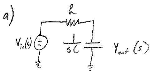
$$V_{out}(s) = V_{in}(s) \frac{\frac{1}{sC}}{R + \frac{1}{sC}} = \frac{1}{RCs + 1}$$
