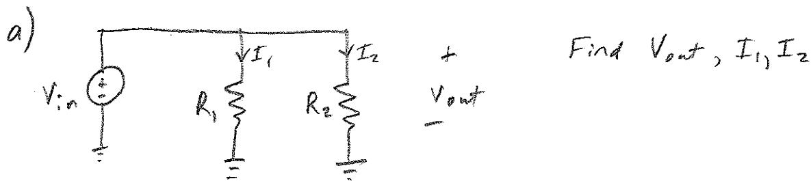
$V_{out} = V_{in} = 1\text{ V}$   $\rightarrow R_1$  and  $R_2$  are in parallel with the voltage source
