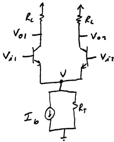
For  $A_{dm} \rightarrow$  Differential Half Mode Circuit
