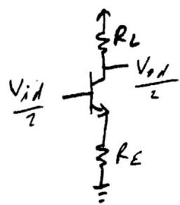
$$A_{dm} = \frac{-\beta R_L}{r_\pi + (1+\beta)(R_E)}$$
