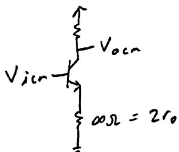
$$A_{cm} = \frac{-\beta R_L}{\frac{2 + V_T}{\alpha I_b} + (1 + \beta)(2 r_o)} = \boxed{0} \quad r_o \rightarrow \infty$$
