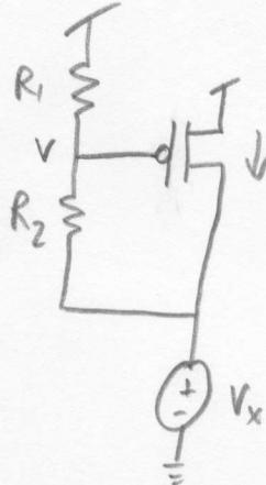
$$V = V_{dd} \frac{R_2}{R_1 + R_2} + V_x \frac{R_1}{R_1 + R_2}$$
