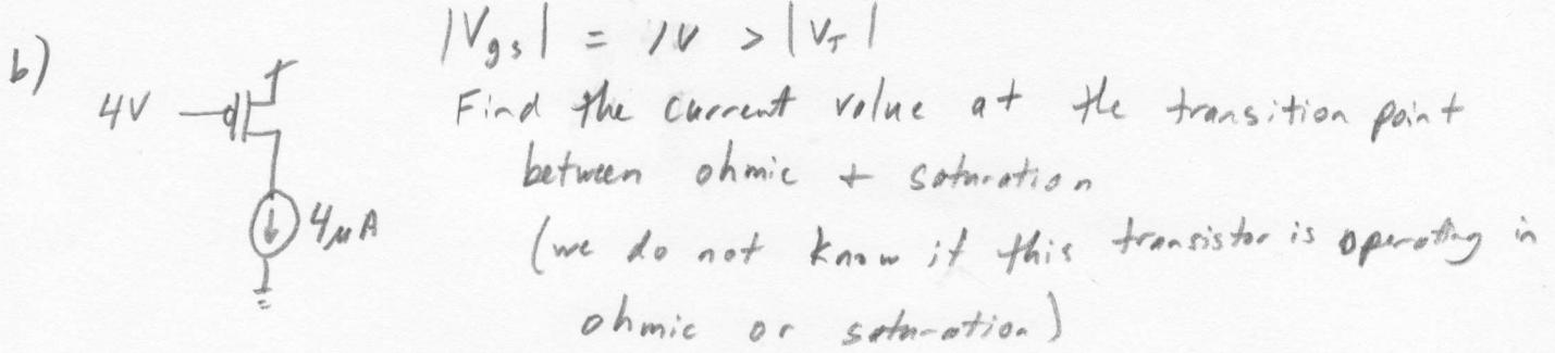
$$I = \frac{K}{2} (|V_{gs}| - V_T)^2 = \frac{100\mu A/V^2}{2} (0.3V)^2 = 4.5\mu A$$
