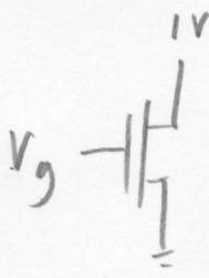
This needs to be operating in above  $V_T$  to generate this resistance ( $V_{ds} = 1\text{V} \rightarrow$  will not be able to be sub  $V_T$  ohmic)
