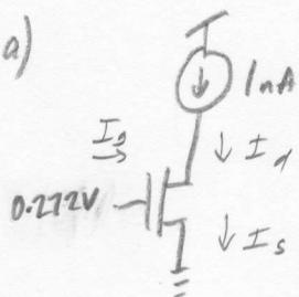
$$V_g - V_s = 0.275V < V_T \Rightarrow \text{sub } V_T \text{ operation}$$
