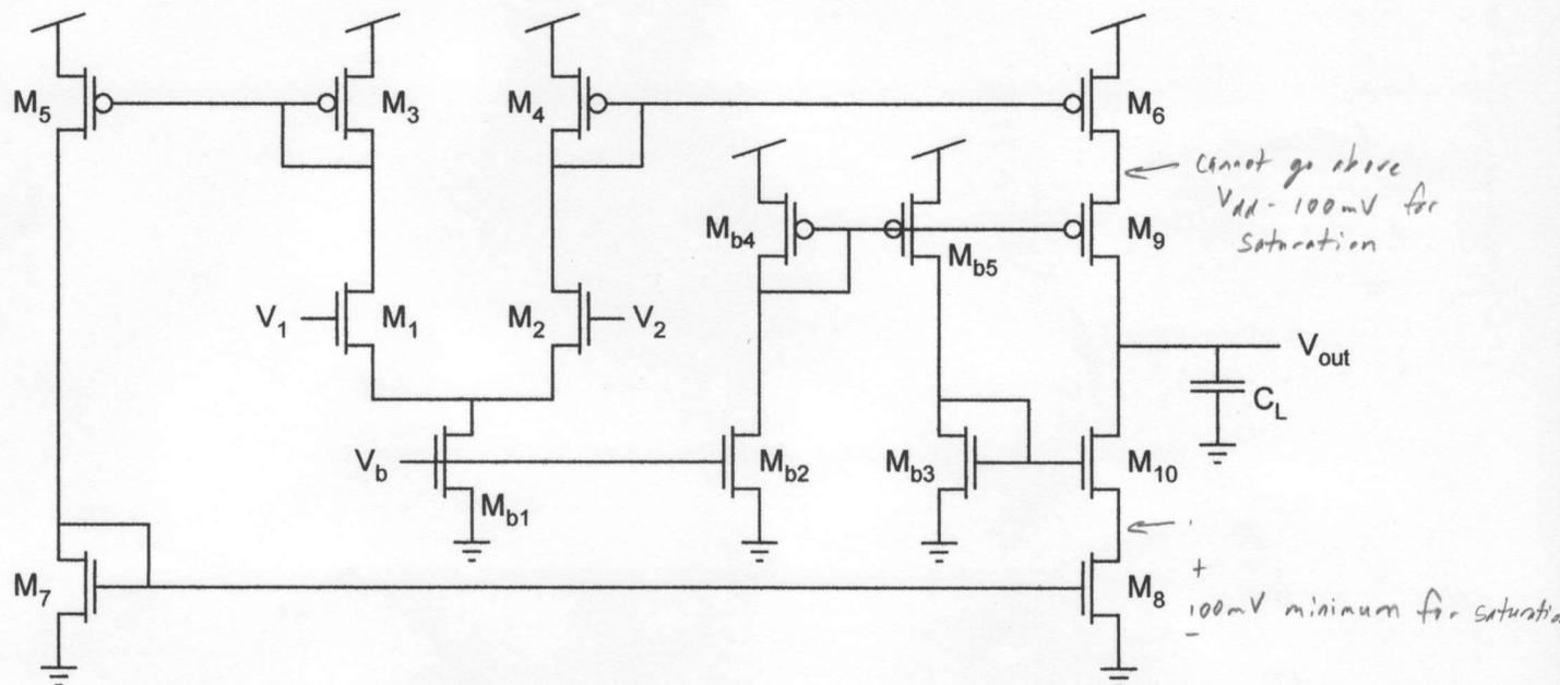
$$R_{out} = r_{o6} g_{m9} r_{o9} \parallel r_{o8} g_{m10} r_{o10} \quad g_{m9} = g_{m10} = |g_{m1}| = \frac{I_{b1}}{V_T} = \frac{50\text{nA}}{25.9\text{mV}} = 1.93\mu\text{S}$$
