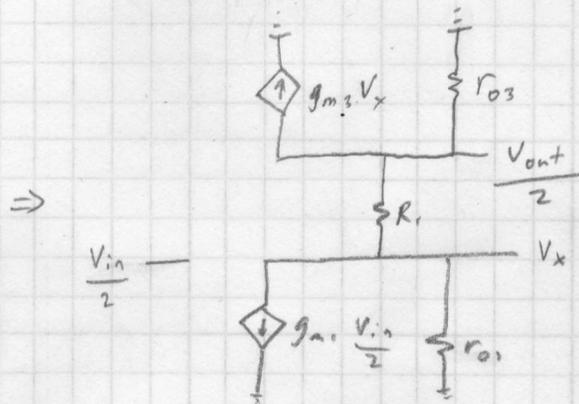
$$\text{KCL at } V_x \rightarrow \frac{1}{2}g_{m1}V_{in} + \frac{V_x}{r_{o1}} + \frac{V_x - \frac{V_{out}}{2}}{R_1} = 0 \Rightarrow \frac{1}{2}g_{m1}V_{in} + V_x \left( \frac{1}{r_{o1}} + \frac{1}{R_1} \right) = \frac{V_{out}}{2R_1}$$
