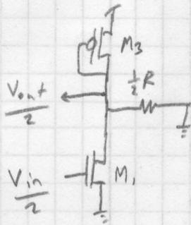
$$a_v = -g_{m1} r_{o1} \parallel r_{o3} \parallel \frac{1}{2}R \parallel \frac{1}{g_{m3}}$$
