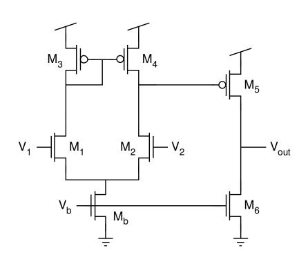
$$A_{v} = (g_{m1}r_{o2} \parallel r_{o4})(g_{m5}r_{o5} \parallel r_{o6})$$
