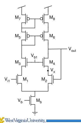
For M<sub>2</sub> and M<sub>4</sub> to stay in saturation
