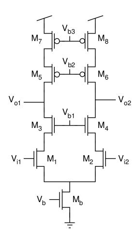
$$A_{v} = g_{m1} (r_{o2} g_{x4} r_{o4} \parallel r_{o8} g_{x6} r_{o6})$$
