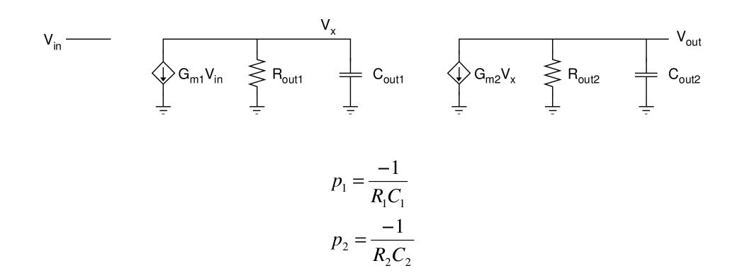
p<sub>2</sub> typically dominates because of the load capacitance
