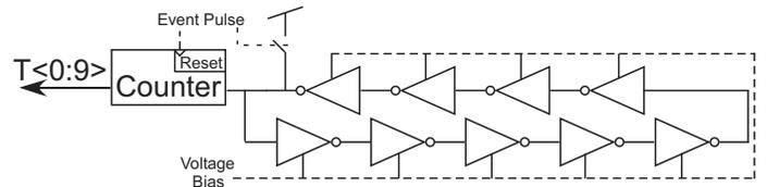
Fig. 5. Time-to-digital converter consisting of a voltage-controlled oscillator and a counter. The counter keeps track of the number of oscillations. The resulting digital word is proportional to the time elapsed since the last event pulse. The event pulse clears the counter and also shorts part of the oscillator to logic high, which ensures that it begins in the same state after every reset.
