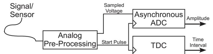
Fig. 1. Asynchronous analog-to-digital conversion system. A reconfigurable analog front end reduces information to only the relevant data points and also triggers the subsequent blocks which then produce digital words for the corresponding voltages and time intervals.
