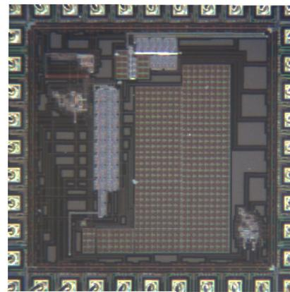
Fig. 2. Die photograph of the asynchronous ADC/TDC fabricated in a  $0.5\mu\text{m}$  standard CMOS process available through MOSIS.
