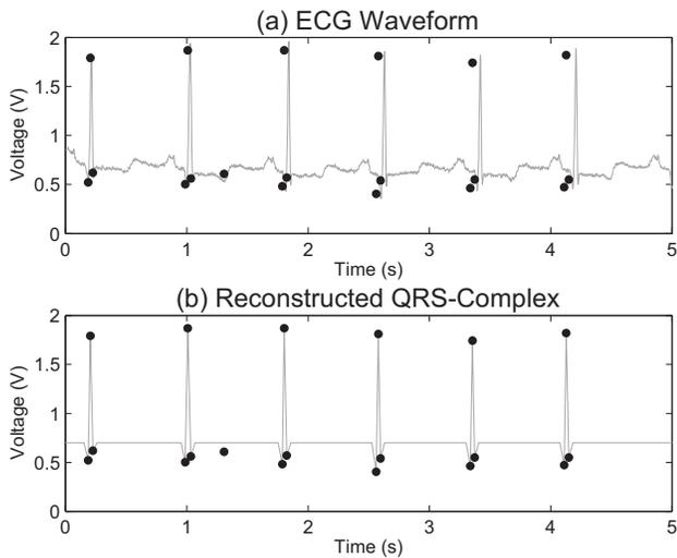
Fig. 6. (a) The original ECG waveform (gray line), taken from the MIT arrhythmia database, with the detected extrema values (black). While the period-to-period temporal accuracy is relatively high, error aggregates creating the appearance of a shorter signal. This aggregate error could be addressed in post-processing. (b) QRS-complex reconstruction (gray) with the detected QRS values (black) as well as a single false positive.
