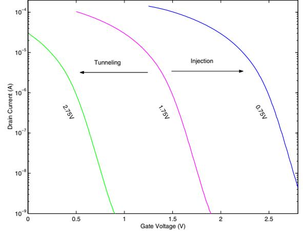
Fig. 2. **Floating-Gate pFET Programming:** Programming a floating-gate transistor using a combination of tunneling and hot-electron injection, the threshold voltage of a pFET is programmed to three different threshold voltages of  $0.75V$ ,  $1.75V$  and  $2.75V$ . The threshold voltage of a non-floating-gate device in the process is approximately  $0.9V$ .
