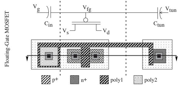
Fig. 1. **Floating-Gate pFET:** Layout and circuit schematic of a floating-gate pFET in a standard double poly n-well CMOS process. External input signals are capacitively coupled onto the floating gate through the input capacitor  $C_{in}$ . The layout shows the realization of  $C_{in}$  using a poly-poly capacitor, although this could also be implemented as a MOS capacitor or a diffused linear capacitor. Between  $V_{tun}$  and the floating gate is the tunneling capacitor  $C_{tun}$ .
