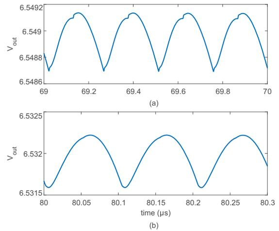
Fig. 5. Simulated ripple for an output voltage of 6.5V with (a)  $0\mu A$  load current and (b)  $20\mu A$  load current.
