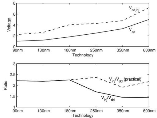
Fig. 1. (Top) Scaling of critical programming voltages: the core supply voltage ( $V_{dd}$ ) and the write (i.e. injection) voltage ( $V_{sd,inj}$ ), (Bottom) Ratio of the write ( $V_{sd,inj}$ ) voltage to the core supply voltage.
