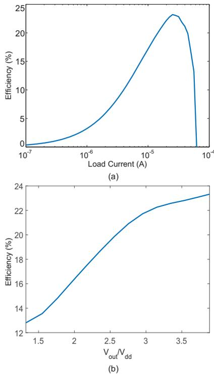
Fig. 4. (a) Measured efficiency of the charge pump versus load current when  $V_{out} = 6.5V$  (b) Measured efficiency of the charge pump versus  $V_{out}/V_{dd}$  for  $20\mu A$  of load current.
