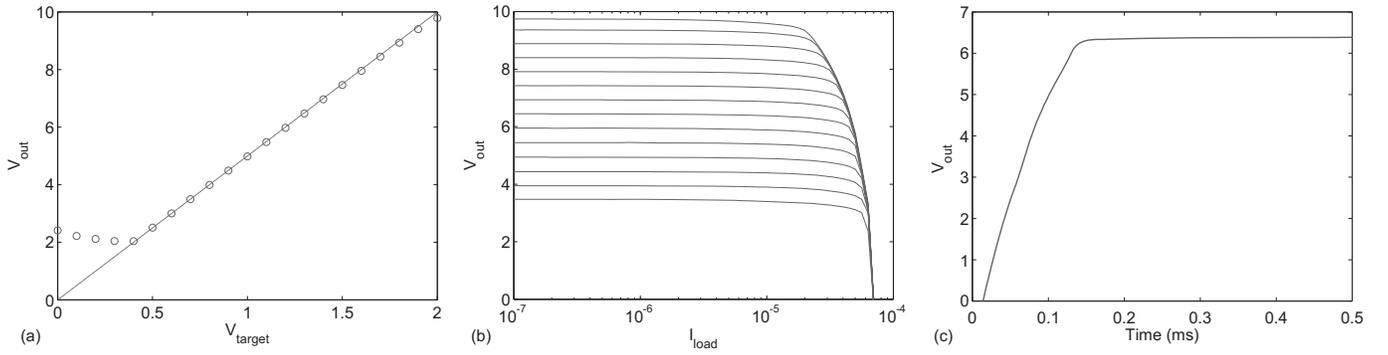
Fig. 3. (a) Measured DC dependence of the charge-pump output on  $V_{target}$  for a purely capacitive load. (b) Measured load regulation of the closed-loop charge pump for various output voltages (c) Measured transient response of the closed-loop charge pump for a  $20\mu A$  load current.
