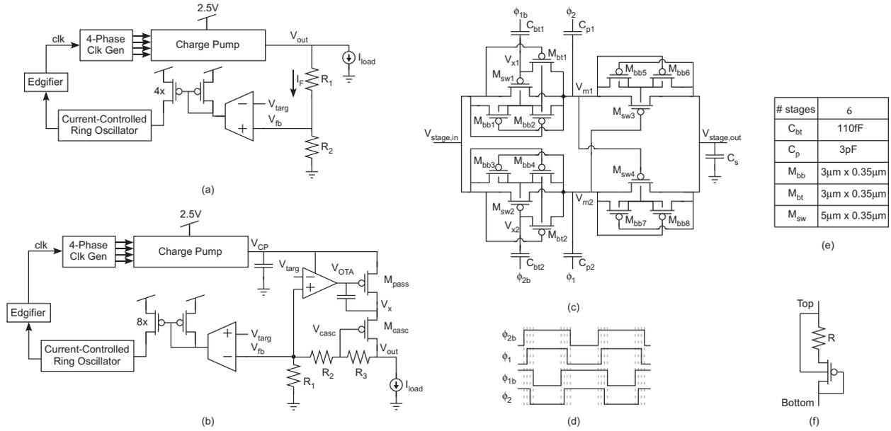
Fig. 2. (a) Block diagram of tunneling charge pump we presented in [3]. (b) Block diagram of the proposed injection charge pump. (c) Circuit diagram of the charge transfer switch (CTS). (d) Non-overlapping clock signals necessary for the CTS. (e) Charge pump specifications. (f) Transistor-level details of the resistor cell to implement the resistive divider.
