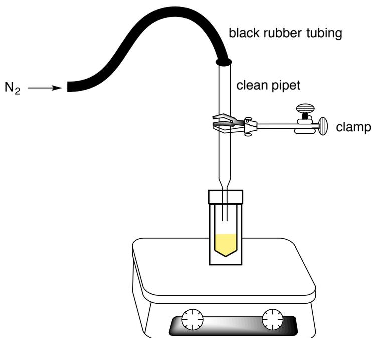
Figure 10. Evaporation Setup
