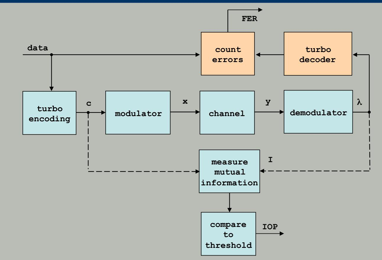
► A fine-grain simulation requires a turbo decoder.
