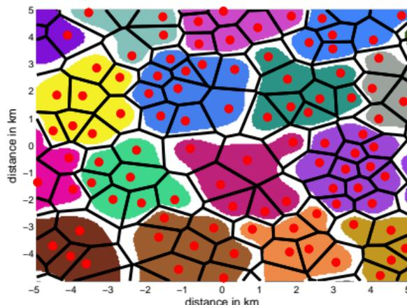
**Figure:** Close-up of an example network topology. The white areas are the portion of the network for which the outage probability is above a typical value of  $\hat{\epsilon} = 0.1$ .
