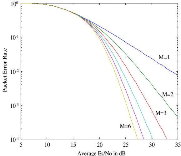
Fig. 3. Average packet error rate of macrodiversity combining in quasi-static Rayleigh fading when MS at location B and the Bluetooth DH5 packet is used.
