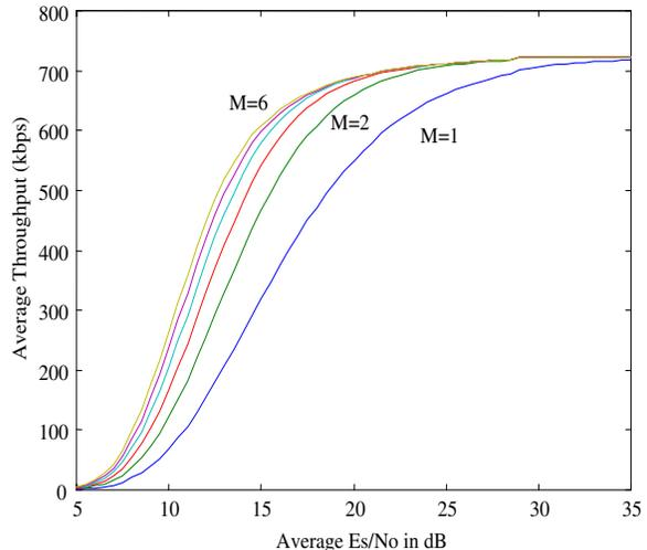
Fig. 6. Average throughput of macrodiversity combining in quasi-static Rayleigh fading when MS at location A, the Bluetooth DH5 packet is used, and the return channel is imperfect.
