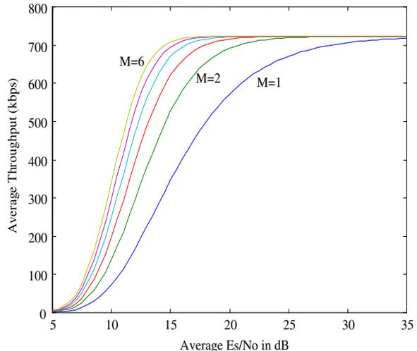
Fig. 4. Average throughput of macrodiversity combining in quasi-static Rayleigh fading when MS at location A, the Bluetooth DH5 packet is used, and a perfect ARQ return channel is assumed.
