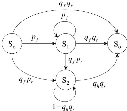
Fig. 5. State diagram representation of Bluetooth stop-and-wait ARQ protocol using macrodiversity reception.
