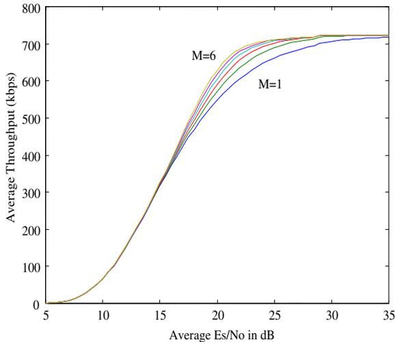
Fig. 7. Average throughput of macrodiversity combining in quasi-static Rayleigh fading when MS at location B, the Bluetooth DH5 packet is used, and the return channel is imperfect.
