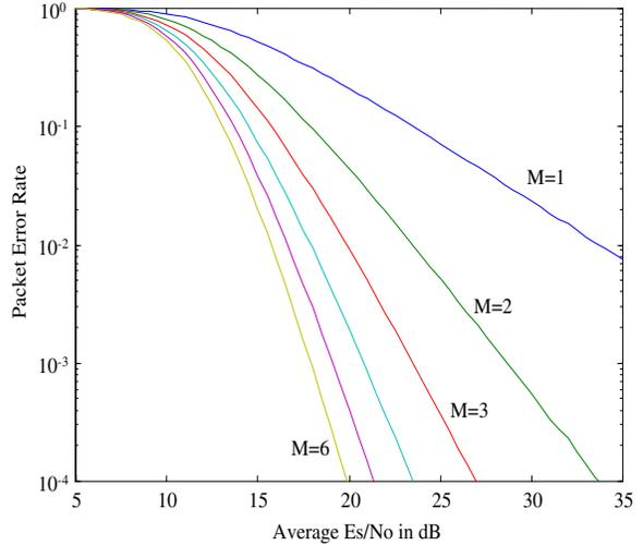
Fig. 2. Average packet error rate of macrodiversity combining ( $M$  APs) in quasi-static Rayleigh fading when MS at location A and the Bluetooth DH5 packet is used.
