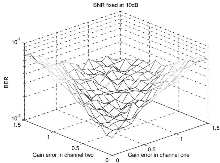
Figure 6. Performance of STBC in Rayleigh flat fading with QPSK modulation, two transmit antennas, one receive antenna, a **fixed SNR of 10 dB**, and a maximum gain error of **1.5**.
