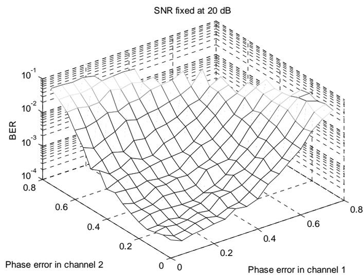
Figure 4. Performance of STBC in Rayleigh flat fading with QPSK modulation, two transmit antennas, one receive antenna, a **fixed SNR of 20 dB**, and a maximum phase error of  $\pi/4$  radians.
