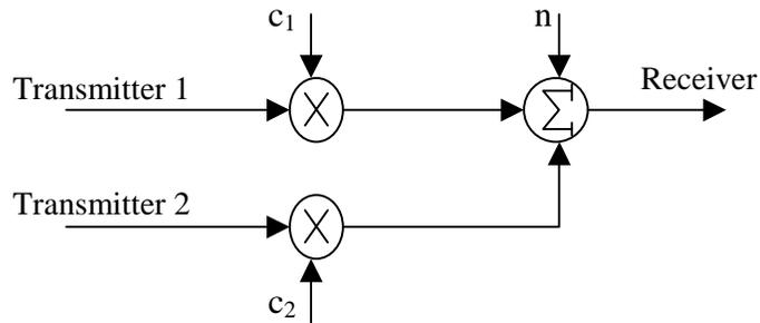
Figure 1: Transmission system consisting of two transmit antennas and one receive antenna.
