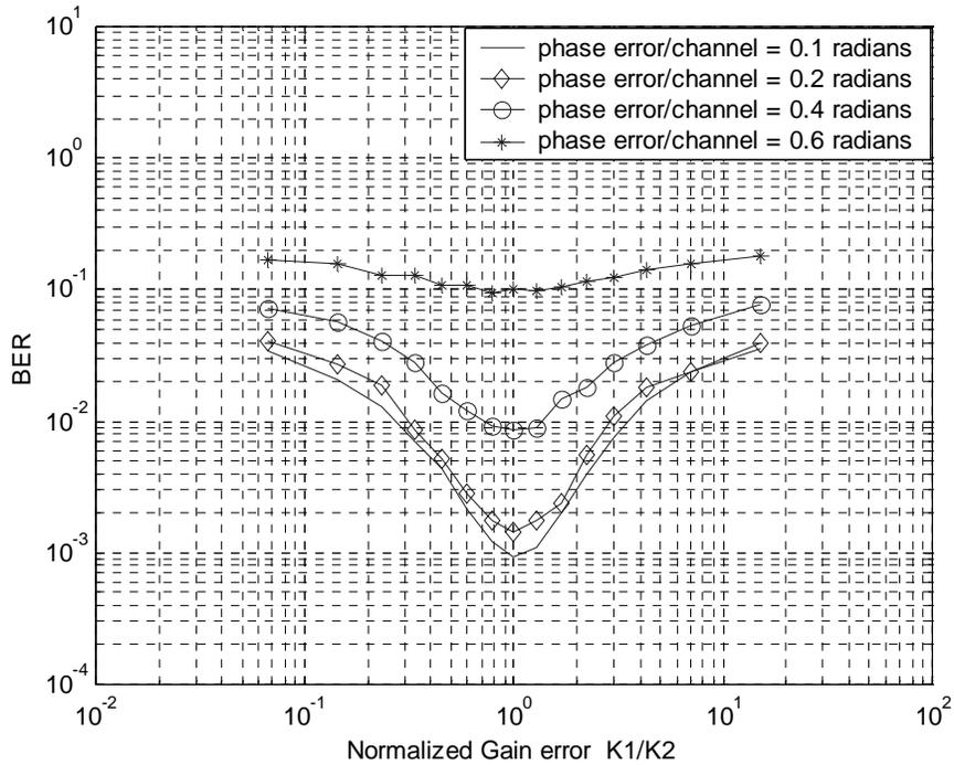
Figure 11. BER versus normalized gain error for STBC in Rayleigh flat fading with QPSK modulation, two transmit antennas, one receive antenna, a fixed SNR of 20 dB and various levels of phase errors per channel.
