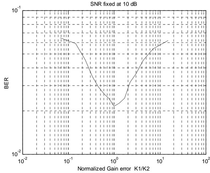
Figure 7. Performance of STBC in Rayleigh flat fading with QPSK modulation, two transmit antennas, one receive antenna, a **fixed SNR of 10 dB**, and **a range of gain error**.
