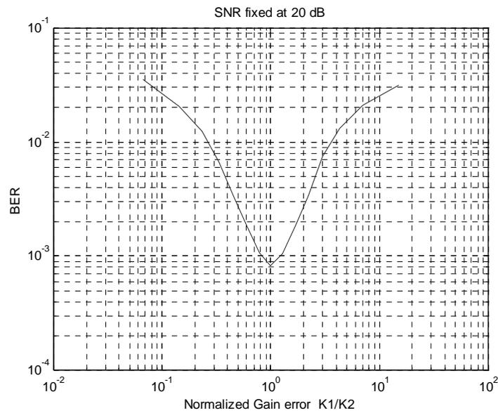
Figure 8. Performance of STBC in Rayleigh flat fading with QPSK modulation, two transmit antennas, one receive antenna, a **fixed SNR of 20 dB**, and **a range of gain error**.
