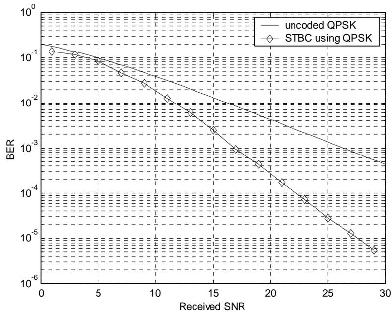
Figure 2. Performance of STBC in Rayleigh flat fading with QPSK modulation, perfect CSI, two transmit antennas, and one receive antenna.
