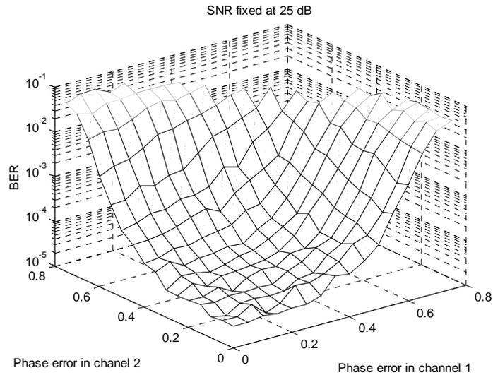
Figure 5. Performance of STBC in Rayleigh flat fading with QPSK modulation, two transmit antennas, one receive antenna, a **fixed SNR of 25 dB**, and a maximum phase error of  $\pi/4$  radians.
