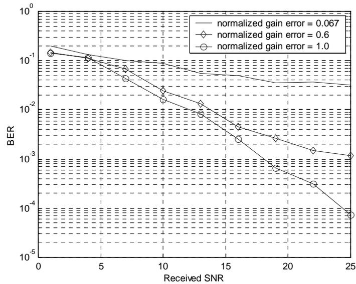
Figure 10. Performance of STBC in Rayleigh flat fading with QPSK modulation, two transmit antennas, one receive antenna, and **various levels of gain errors per channel.**
