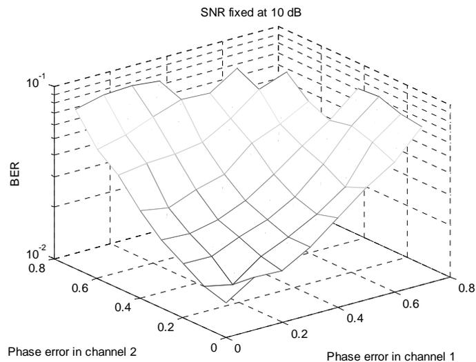
Figure 3. Performance of STBC in Rayleigh flat fading with QPSK modulation, two transmit antennas, one receive antenna, a **fixed SNR of 10 dB**, and a maximum phase error of  $\pi/4$  radians.
