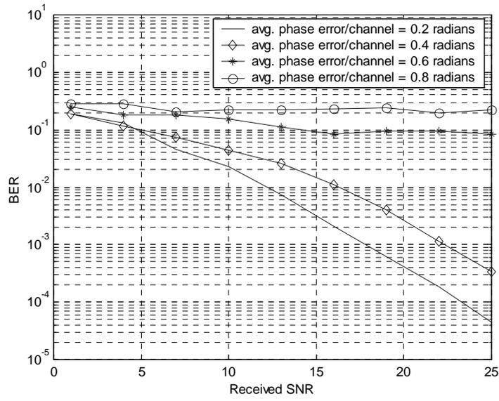
Figure 9. Performance of STBC in Rayleigh flat fading with QPSK modulation, two transmit antennas, one receive antenna, and **various levels of phase errors per channel.**
