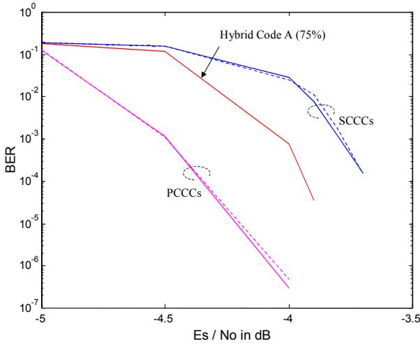
Figure 8: BER performance comparison of  $r = \frac{1}{3}$  PCCC, SCCC and hybrid codes with frame size = 4096 bits vs.  $E_s/N_0$  in dB.
