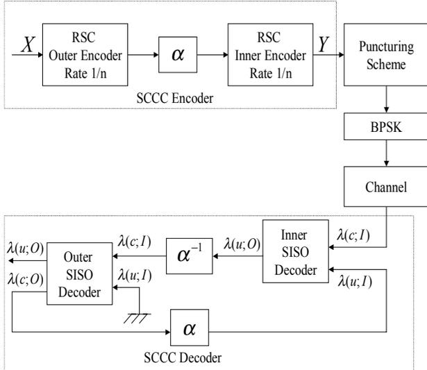
Figure 1: System model of a parent SCCC code.
