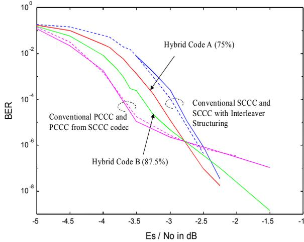
Figure 5: BER performance comparison of  $r = \frac{1}{3}$  PCCC, SCCC and hybrid codes with frame size = 512 bits vs.  $E_s/N_0$  in dB.
