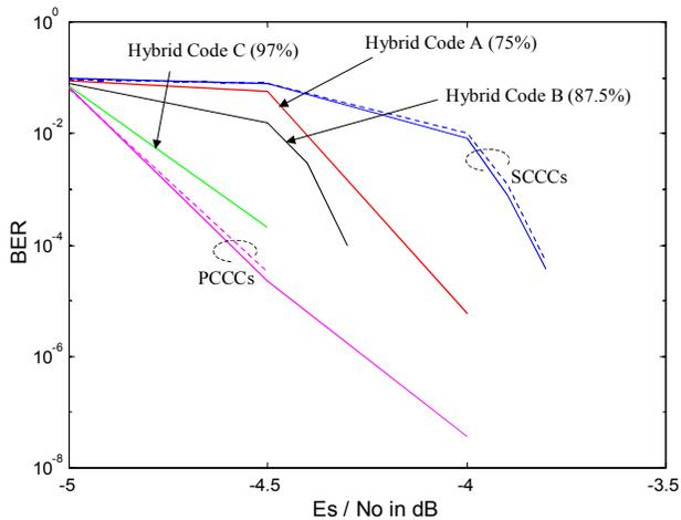
Figure 9: BER performance comparison of  $r = \frac{1}{3}$  PCCC, SCCC and hybrid codes with frame size = 8192 bits vs.  $E_s/N_0$  in dB.
