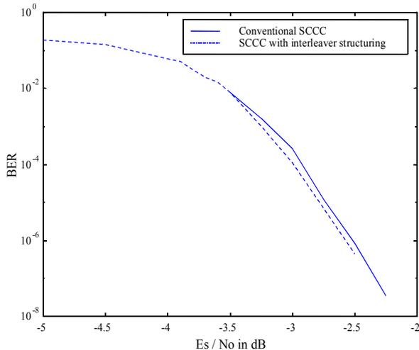
Figure 2: Performance comparison of a  $r = \frac{1}{3}$  SCCC code with and without interleaver structuring.
