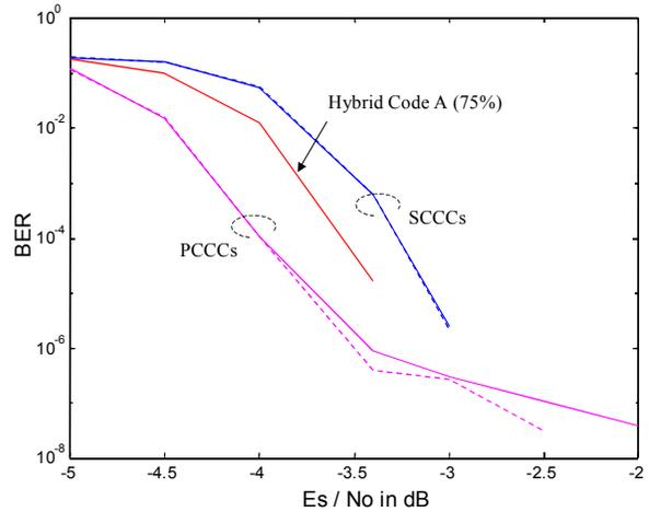
Figure 6: BER performance comparison of  $r = \frac{1}{3}$  PCCC, SCCC and hybrid codes with frame size = 1022 bits vs.  $E_s/N_0$  in dB.
