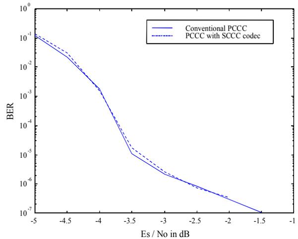
Figure 4: Performance comparison of a conventional  $r = \frac{1}{3}$  PCCC and a PCCC generated by puncturing all the double parity bits of an equivalent  $r = \frac{1}{3}$  SCCC codec.
