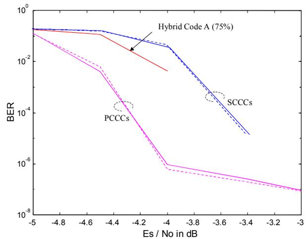
Figure 7: BER performance comparison of  $r = \frac{1}{3}$  PCCC, SCCC and hybrid codes with frame size = 2048 bits vs.  $E_s/N_0$  in dB.
