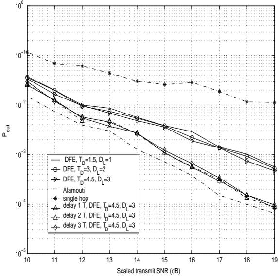
Figure 3: Comparison of Protocol 1 with that of [5] employing an Alamouti code. The pathloss coefficient  $\mu = 3$ . The number of nodes in an area is  $K + 2 = 100$ . Recall that  $D_L$  is the length of one side of the square region considered.  $T_D$  is the maximum propagation delay in the region in terms of the number of symbol periods. Curves labeled with “delay  $nT$ ” correspond to Variant B of Protocol 1, while those without such a label correspond to Variant A.
