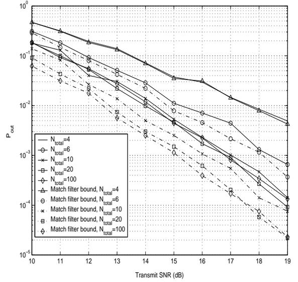
Figure 5: Performance of Protocol 2, Variant A with normalization of the received noise power. In simulations, the parameters are set as  $\mu = 0$ ,  $D_L = 3$ ,  $T_D = 4.5T$ .
