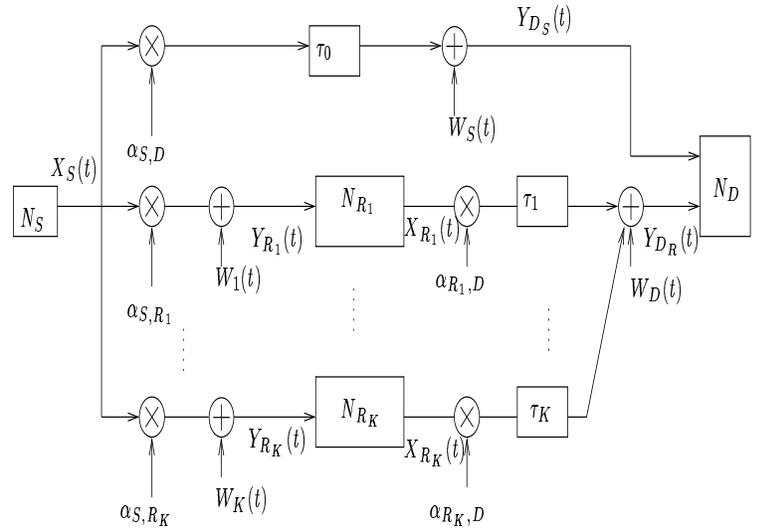
Figure 1: System model of an ad hoc wireless network
