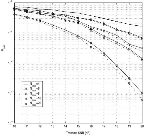
Figure 4: Performance of Protocol 2, Variant A without normalization of the received noise power. In simulations, the parameters are set as  $\mu = 3$ ,  $D_L = 3$ ,  $T_D = 4.5T$ .
