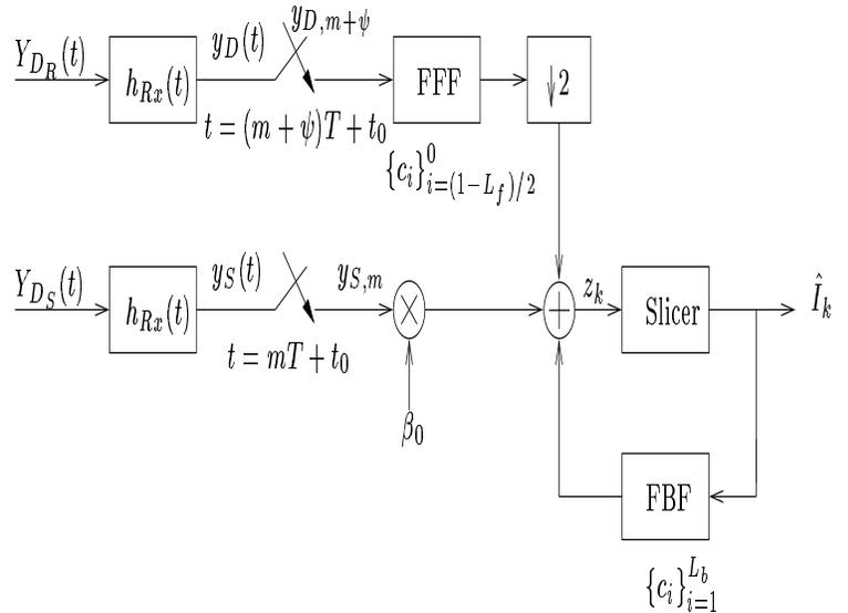
Figure 2: Functional description of the generalized DFE receiver. The signal  $Y_{D_S}(t)$ , and hence  $y_{S,m}$ , is collected by the receiver while the source is transmitting, and the signal  $Y_{D_R}(t)$ , and hence  $y_{D,m+\psi}$ , is collected by the receiver while the relays are transmitting, and then both are processed jointly.
