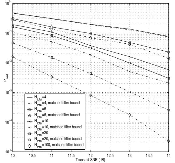
Figure 6: Performance of Protocol 2, Variant B with normalization of the received noise power. In simulations, the parameters are set as  $\mu = 0$ ,  $D_L = 3$ ,  $T_D = 4.5T$ . The pool of delays is  $\{T, 2T, \dots, 6T\}$  from which delays are randomly allocated to the packets transmitted by the active relays.
