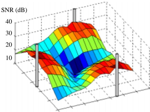
Fig. 5: SNR required for  $BER \leq 10^{-3}$  for 120-degree sectorized antennas as function of mobile's location in the area given by Fig. 4. Base station locations are indicated by vertical bars.
