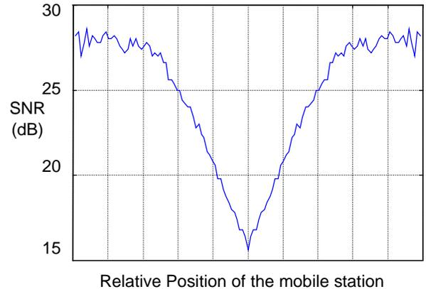
Fig. 3: SNR required for  $BER < 10^{-3}$  as function of mobile's location between two base stations. Base stations are located at the left and right edges of plot.
