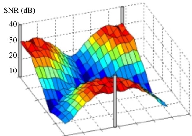
Fig. 7: SNR required for  $BER \leq 10^{-3}$  for 60-degree sectorized antennas as function of mobile's location in the area given by Fig. 6. Base station locations are indicated by vertical bars.
