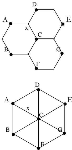
Fig. 8: Topology of 120-degree sectorized system (top) and 60-degree sectorized system (bottom).
