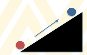
A hot ball at rest at the bottom of a hill does not start moving uphill, while cooling down.
