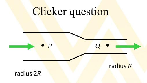
An incompressible fluid flows through a pipe of varying radius (shown in cross-section). Compared to the fluid at point P, the fluid at point Q has
