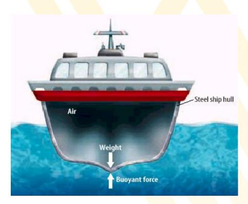
The hull contains mostly air and displaces a lot of water...enough so that  $F_b = F_g$  and it floats.
