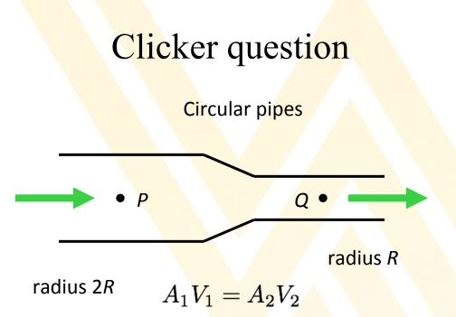
A fluid flows through a pipe of varying radius (shown in cross-section). Compared to the fluid at point P, the fluid at point Q has
