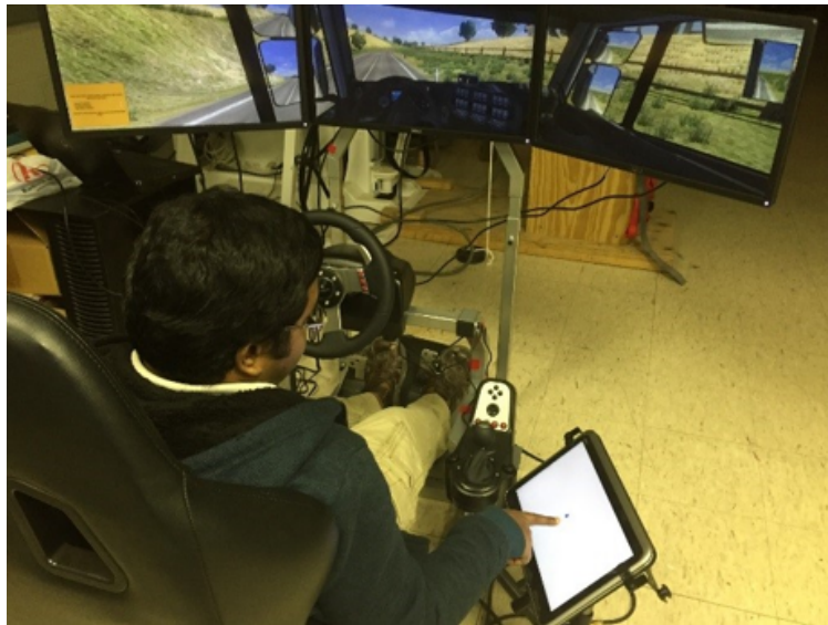
Fig 6 Driving simulator used for data collection. The three monitors present the road view to the driver. The tablet represents the console interface operated by the driver. This setup emulates the cabin inside haul trucks at surface mines.
