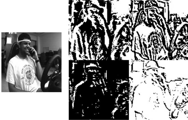
Fig 2 Illustration of the convolution operations (using a few convolution filters) on image data
