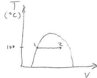
Solution:  $Q - W = m((u_2 - u_1) + \cancel{\frac{V_2^2 - V_1^2}{2}} + g(z_2 - z_1))$
