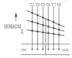
Observe that each temperature profile is a straight line and that the gradient of the line increases with increase in heat flow. Calculate the gradient of each line and show that  $\frac{Q}{\text{gradient}}$  is a constant (C).
