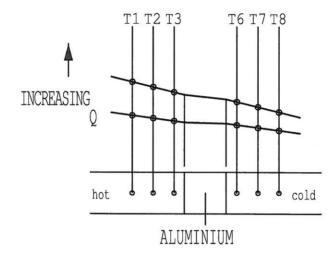
Observe the temperature gradient decreases in the aluminium section because of the increased thermal conductivity of the material (reduced resistance to heat flow). Measure the temperature gradient through the aluminium section from the graph then calculate the thermal conductivity using the average gradient. Compare the value obtained with that previously calculated.
