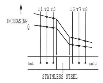
Observe that the temperature gradient increases in the Stainless Steel section because of the reduced thermal conductivity of the material (increased resistance to heat flow).
