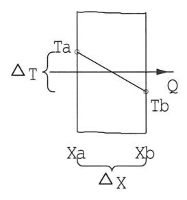
According to Fourier's law of heat conduction:
