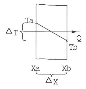
According to Fourier's law of heat conduction:
