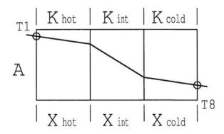
For continuity, the steady heat flow through the successive sections must be the same so Fourier's Law can be applied to the three sections as follows:
