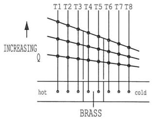
Observe that each temperature profile is a straight line and that the gradient of the line increases with increase in heat flow.
