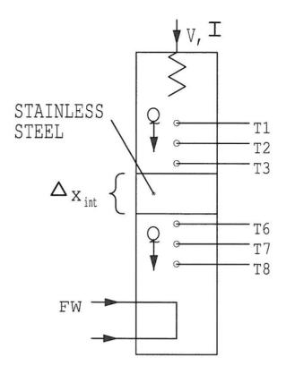
• Connect the eight thermocouples on the HT11C (3) to the appropriate sockets on the front of the service unit (30). Ensure that the labels on the thermocouple leads (T1 - T8) match the labels on the sockets.
