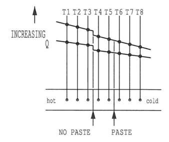
Observe that a step change in temperature occurs at both joints due to the poor thermal contact.
