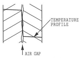
Air trapped in the gaps between each surface acts as an insulator resulting in a temperature gradient in the conduction path. This can be reduced by the use of thermal paste which fills the air spaces and provides thermal contact.
