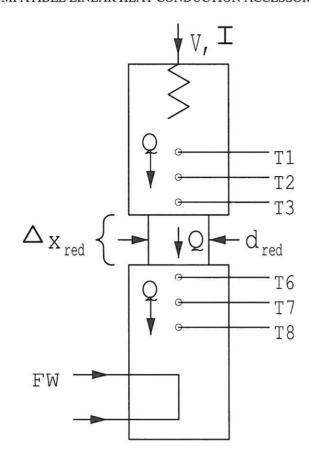
• Connect the eight thermocouples on the HT11C (3) to the appropriate sockets on the front of the service unit (30). Ensure that the labels on the thermocouple leads (T1 - T8) match the labels on the sockets.
