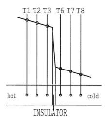
Observe that the temperature gradient in the two brass sections is the same and extremely small because of the low heat flow.
