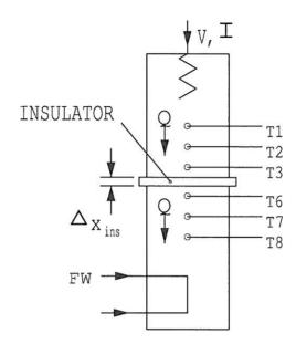
• Connect the eight thermocouples on the HT11C (3) to the appropriate sockets on the front of the service unit (30). Ensure that the labels on the thermocouple leads (T1-T8) match the labels on the sockets.
