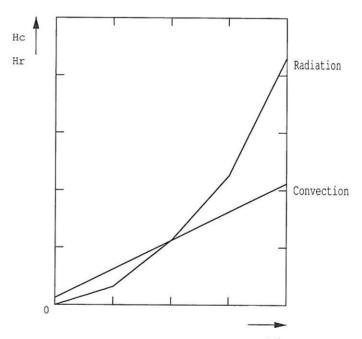
Observe that at low surface temperatures (typically less than 230°C) the heat transfer coefficient  $H_{cm}$  due to natural convection is greater than the heat transfer coefficient  $H_{rm}$  due to radiation. Conversely, at high surface temperatures (typically greater than 230°C) the heat transfer coefficient  $H_{cm}$  due to natural convection is less than the heat transfer coefficient  $H_{rm}$  due to radiation and as the temperatures exceeds 400°C the effect of radiation becomes dominant.
