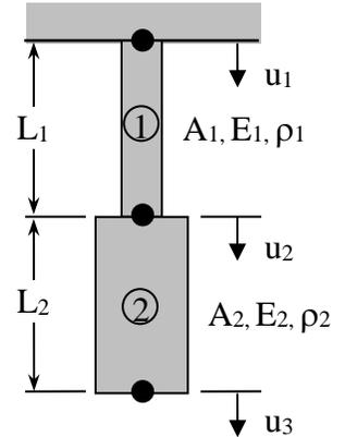
$$\begin{aligned}L_1 &= L_2 = 1 \text{ m} \\A_1 &= 0.001 \text{ m}^2 \\A_2 &= 0.004 \text{ m}^2 \\E_1 &= E_2 = 70 \times 10^9 \text{ Pa} \\ \rho_1 &= \rho_2 = 2700 \text{ kg/m}^3\end{aligned}$$
