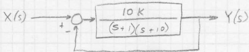
Next, reduce the feedback connection, with the feedback gain of 1
