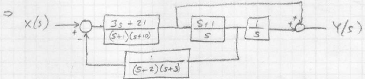
Move one connection to create a feedback loop and a parallel connection
