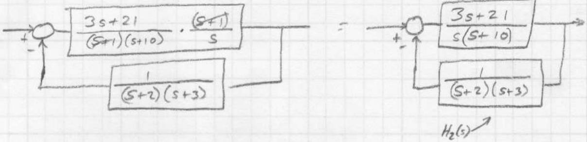
$$F.B. = \frac{H_1(s)}{1 + H_1(s) H_2(s)} = \frac{\frac{3s+21}{(s+1)(s+10)} \cdot \frac{(s+1)}{s}}{1 + \frac{3s+21}{s(s+10)}} =$$
