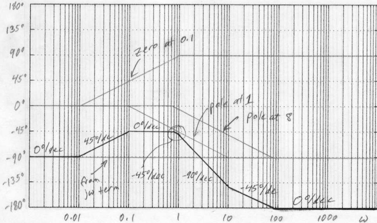
Three poles and one zero  $\rightarrow$  as  $\omega \rightarrow \infty$ ,  $\angle H(j\omega) = -180^\circ$
