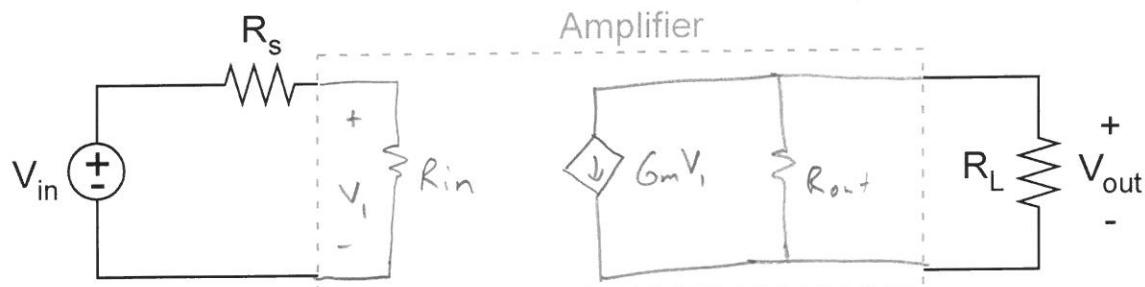
$$V_i = V_{in} \frac{R_{in}}{R_{in} + R_s}$$
