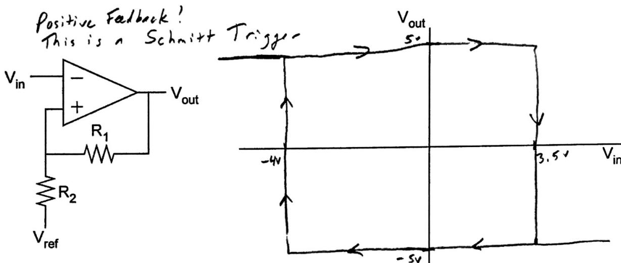
$V_{out}$  can be either  $\pm V_{sat} = \pm 5V$
