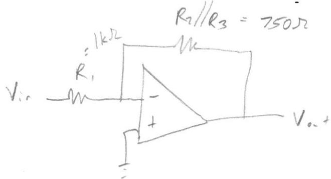
$$\frac{V_{out+}}{V_{in}} = - \frac{R_2 // R_3}{R_1} = - \frac{750\Omega}{1k\Omega} = \boxed{-0.75}$$
