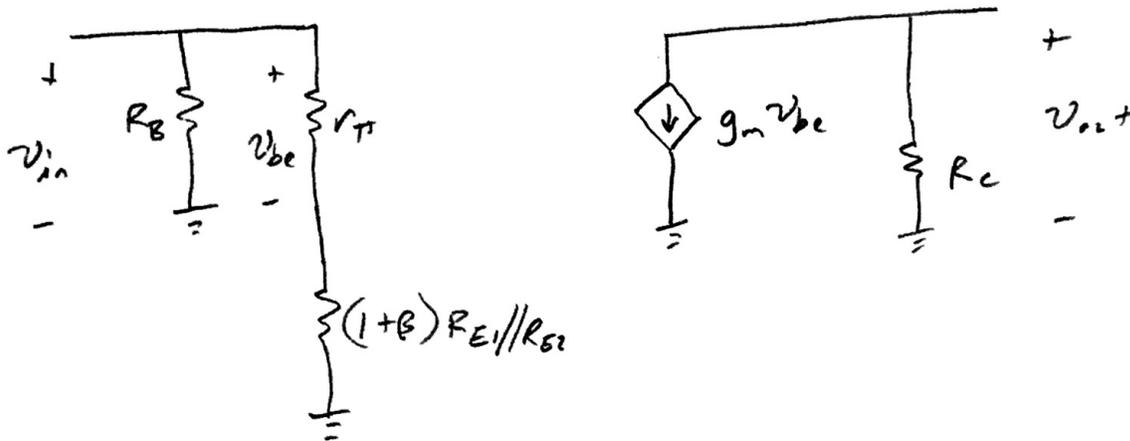
$$v_{out} = -g_m v_{be} R_C$$
