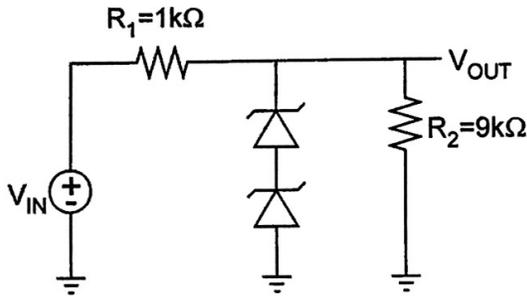
When the Zener diodes are in reverse-b. breakdown,  $V_{out} = 2(5.6V) = 11.2V$
