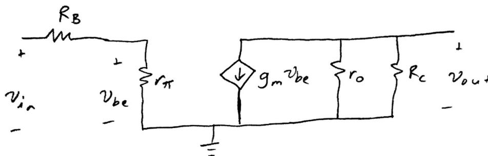
D. Calculate the small-signal voltage gain for this circuit.
