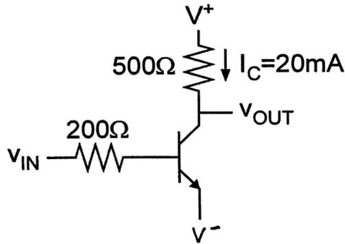
A. Calculate the transconductance of the transistor.
