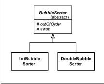
Figure 15-1 Bubble Sorter Structure
