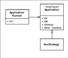
**Figure 15-2** Strategy structure of the Application algorithm.
