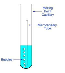
Figure 3. Micro Boiling Point Capillary
