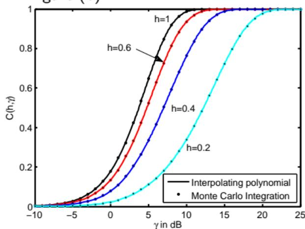
(a) channel capacity versus SNR  $\gamma$
