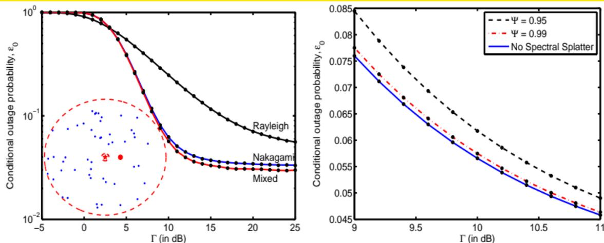
Figure: Conditional outage probability as a function of SNR  $\Gamma$ .
