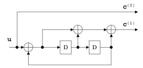
The feedback of one output allows one of the outputs to be the input, hence it is *systematic*.
