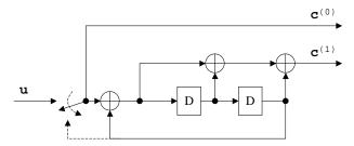
Throwing the switch down after the k data bits have been encoded creates a tail that will bring the encoder back into the all-zeros state.
