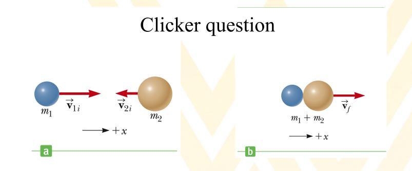
How do you expect the total (kinetic) energy to change in this collision process (one partner initially at rest, partners stick together after collision)?
