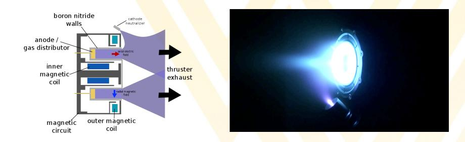
Classical rockets produce a lot of thrust, but cannot be used for small course corrections of e.g. satellites. Plasma thrusters are used instead.
