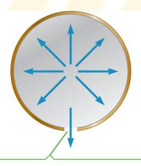
An opening at the bottom of the chamber removes the downward reaction force, resulting in a net upward reaction force.
