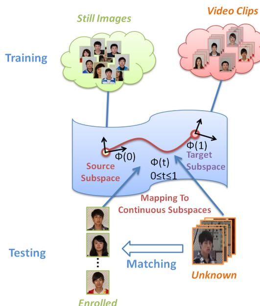
Figure 1. Illustration of the proposed method. In the training stage, still images and video clips are represented as two points on the Grassmann manifold to learn the “transitions” between them. In testing, the still images and video clips are projected on to a sequence of continuous subspaces before matching between them.
